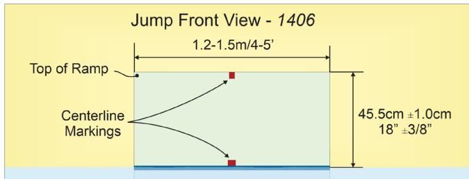
**(B) Surface.** The surface of the ramp out of the water shall be 210cm  $\pm$ 4.2cm long, with the waterline marked by the center of a transverse line of contrasting color of a width equal to the total 8.4cm. The width of the ramp surface shall be a minimum of 1.20m and a maximum of 1.50m ~~with parallel sides~~. The surface of the jump ramp shall be flat with a maximum deviation of  $\pm$ 1cm from a plane. The overall length of the ramp surface shall be a minimum of 3.6m.
